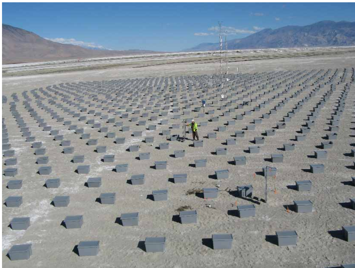
FIGURE 4-10 Test of engineered solid roughness elements at Owens Lake. SOURCE: Holder, 2019d.
