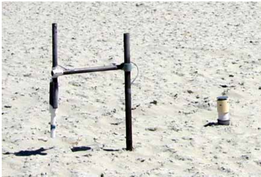
FIGURE 2-7 Photographic image of a Sensit device suspended above the ground (left) and a Cox Sand Catcher (right). NOTE: The Sensit is a battery-powered motion detector used to count sand-sized particles per unit time that saltate (bounce) across the surface. The Cox Sand Catcher is a passive device used to capture samples of windblown, sand-sized particles of dust at a specific height above the surface. SOURCE: Richmond, 2019.
