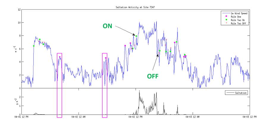
Threshold is defined as the mean of the wind speed at the time the Sensit registers activity and when activity ceases.
