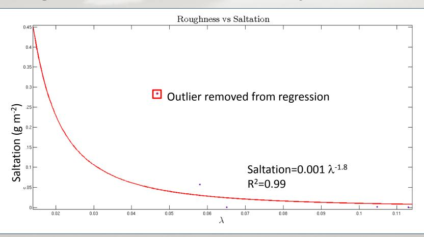
Vegetation effect on sand transport rate (for roughness elements >0.38 m)
