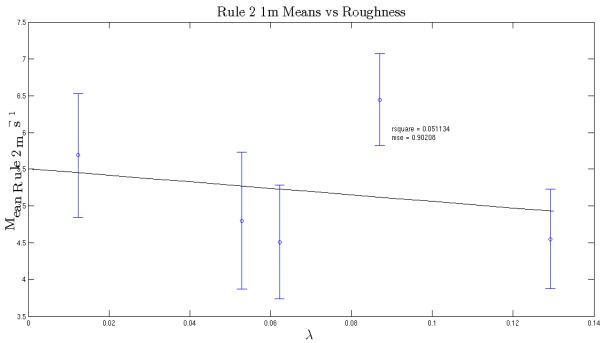
For 1 m wind speed measurements there is too great an effect on local wind speed below the height of the vegetation, which affects the expected relationship (i.e., as  $\lambda$  increases, threshold increases)
