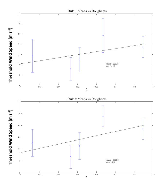
In general an increase in threshold wind speed is observed (for 4 m WS)
