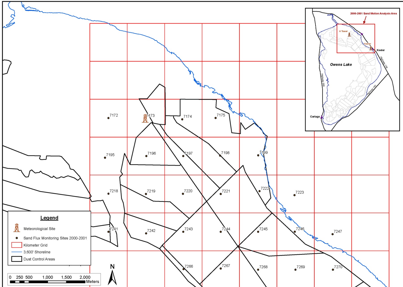
Figure 1. Map showing the kilometer grid and sand motion monitoring sites used in 2000-2001 analysis. Sand motion monitoring sites are labeled by Sensit site number. The dust control areas shown on the map are for reference and were not implemented during the 2000-2001 study period.
