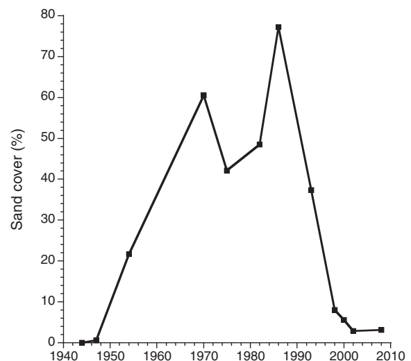
Fig. 15. Variation in sand input to Keeler Dunes over time, as estimated by proportion of sand cover on “Old State Highway” that ran from Keeler to Lone Pine. Secondary peak in cover in 1986 may relate to coverage of highway by dunes.
