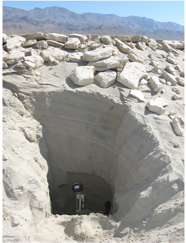
Figure 1 (left). OWN10-2 sampling pit. Metal cans are shown inserted into the wall. The OSL sample was taken with the large can and subsamples for dose-rate determinations correspond to the smaller 1 oz cans.
