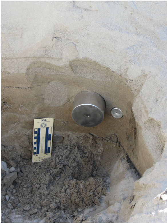
Figure 1 (left). OWN10-2 sampling pit. Metal cans are shown inserted into the wall. The OSL sample was taken with the large can and subsamples for dose-rate determinations correspond to the smaller 1 oz cans.
