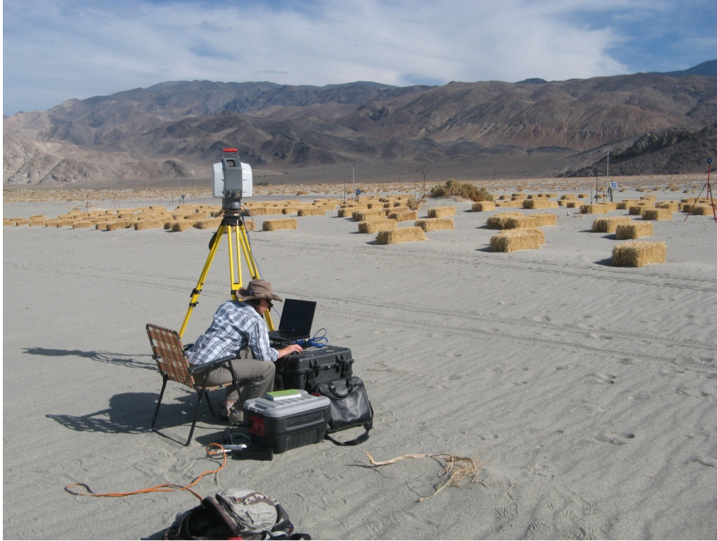
Figure 4. The Terrestrial Lidar Scanner deployed at the Keeler Dunes dust demonstration field site, September 11, 2013.
