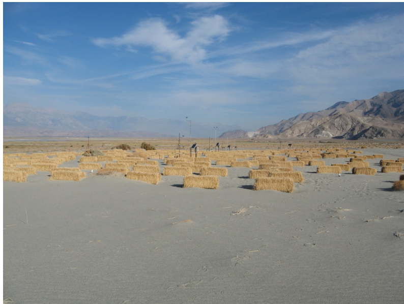
Figure 3. The straw bale roughness elements and the 4 m high meteorological towers with anemometers and wind vanes.
