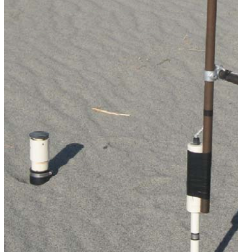
Figure 2. An image of a Cox Sand Catcher (left edge of image) and a Sensit piezoelectric saltation sensor (right edge of image) deployed within the roughness array.
