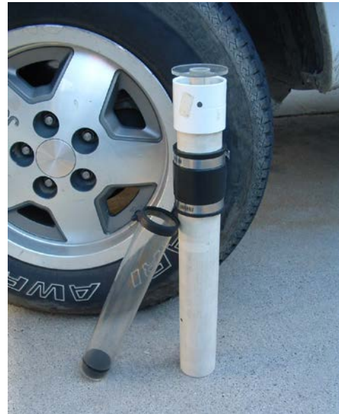
Figure C.2.3 - Example of a Cox Sand Catcher (CSC) with the inner sampling collection tube removed.
