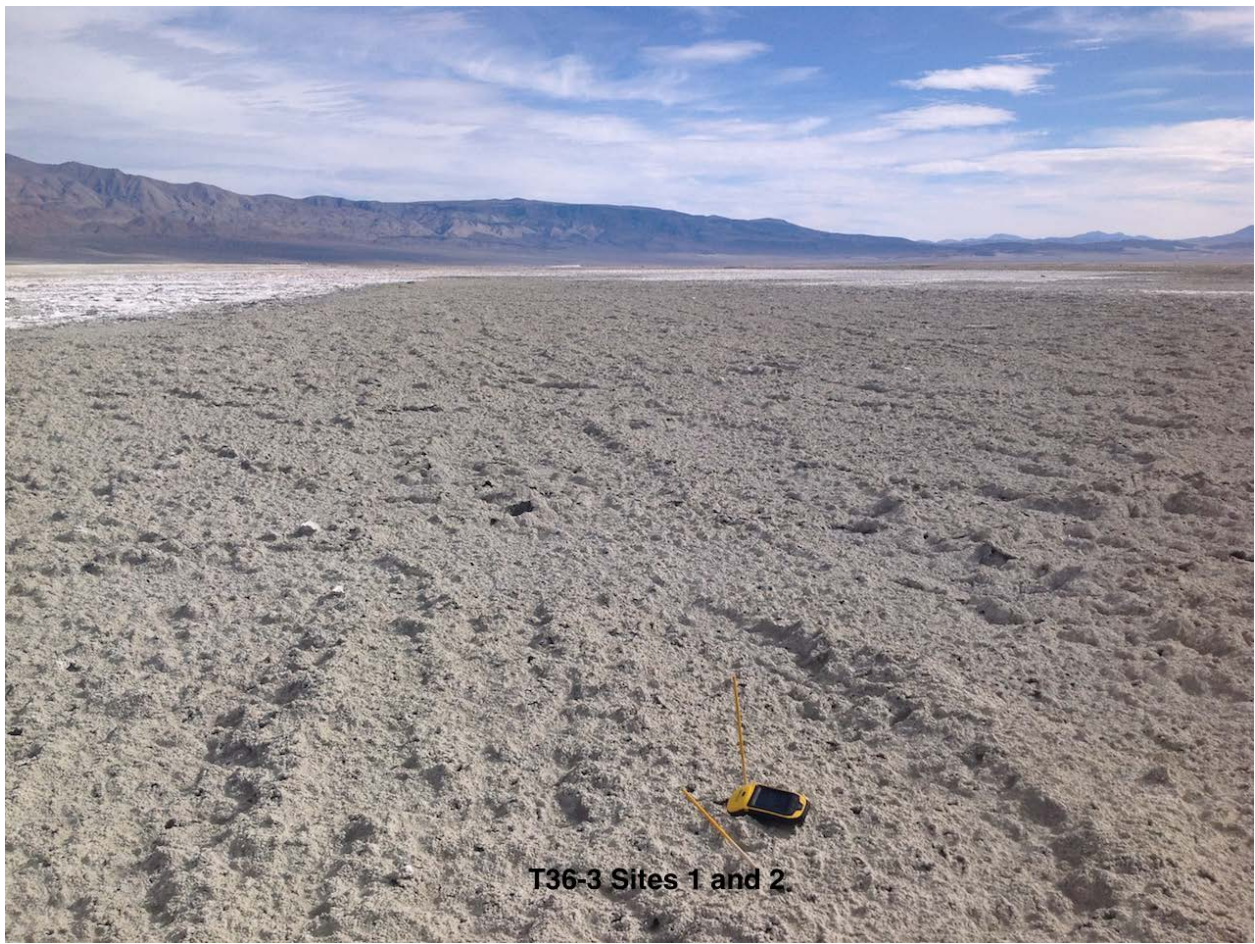
Figure 4. Photo of non-emissive capillary brine salt crust present in the western portion of the T36-3 test area. Crust is located on a slightly elevated portion of the area. The capillary brine crust is 15 to 20 centimeters thick in this area. Note the presence of a mix of open brine and evaporite crust in the upper left.
