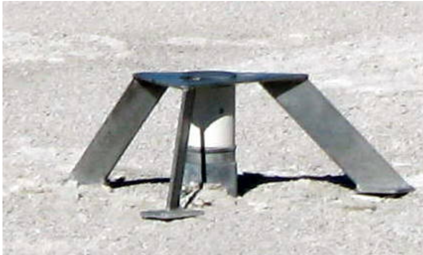
Figure C.2.5 - A Height Adjustment Tool is used to measure the height of Sensits and CSCs and to adjust the sensor and inlet height to 15 cm above the soil surface.
