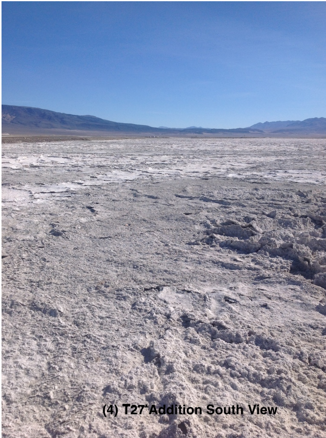
Figure 5. Photo of the T27-Addition test area with thick heaved capillary brine crust in the foreground transitioning to an evaporite salt deposit in the middle of the picture.
