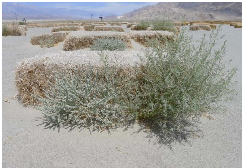
Figure 6-6: Shrubs Planted along the Base of a Straw Bale in the Project Test Site Started in 2013 (20 months after planting)
