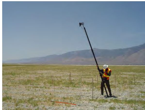
FIGURE A-3 DPF Field Equipment Setup DPF equipment included the use of a high resolution camera mounted on a 15' Hi-Pod monopod.
