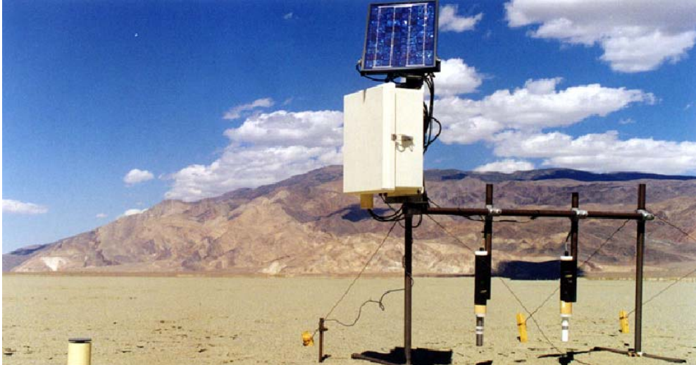
Figure 2.1 Two Sensits are seen suspended above the ground on the right and a CSC is located to the left at this Owens Lake test site used to compare the performance of different saltation measurement instruments.
