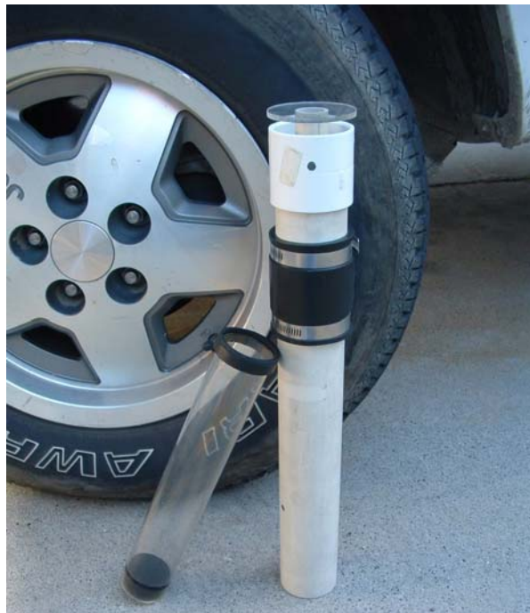
Figure 2.3 Photo of Cox Sand Catcher (CSC) with Inner Sampling Tube Removed
