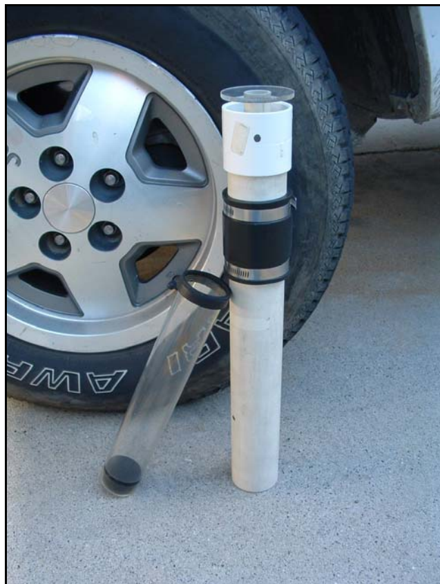
Figure 4.6 – Photo of a Cox Sand Catcher with the inner sampling tube removed.
