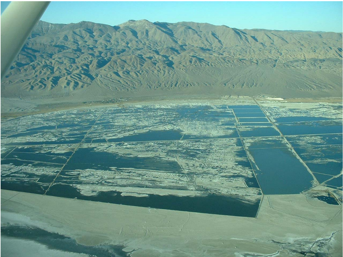
Figure 5.3 – Shallow Flooding – aerial view of sheet flood method (left side of photo)
