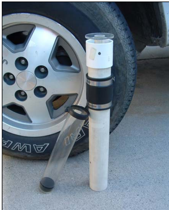
Figure 4.8 – Example of a Cox Sand Catcher (CSC) with the inner sampling tube removed
