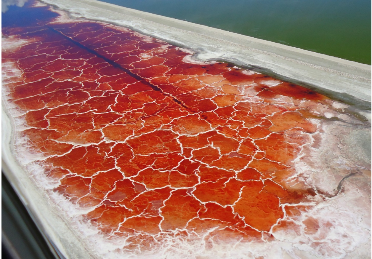
Figure 2. Oblique air photo of T36-3 DCA test area. Open brine is visible as dark red to pink colored areas. White surface is an evaporite crust forming from precipitation of salts from the brine. Heaved pressure ridges in the evaporite crust are visible and divide the brine into a polygonal structure. The width across the dust control cell is approximately 100 meters.
