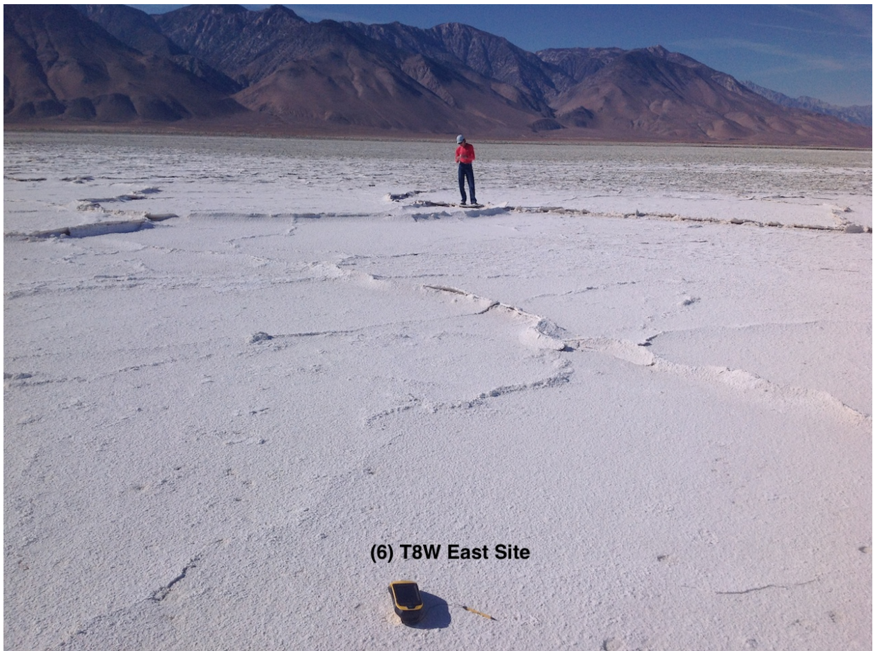
Figure 3. Stable non-emissive evaporite crust formed in T8W DCA test area. Heaved pressure ridges in the evaporite crust create large-scale polygonal structure.
