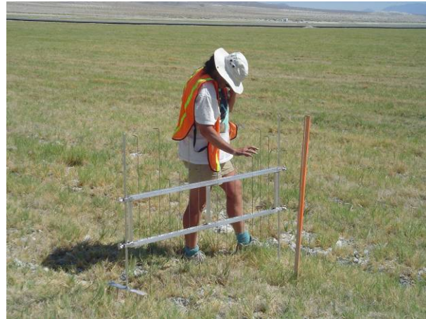
FIGURE A-2 GBUAPCD Point Frame Device The GBUAPCD PF device is approximately 5 feet wide with 14 individual pins.
